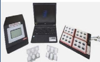
**Study the effects of tension, compression and shear stress on 2D and 3D cell cultures.**
